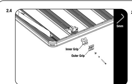
Loosley fit one Inner Grip and one Outer Grip to each Grab On Foot using a M6 Cap Screw, M6 Spring Washer and M6 Washer.
