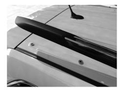
( **B** ) Place a Foam Washer (Item 10), white backing facing up, over each of the bosses on the vehicle's roof.
