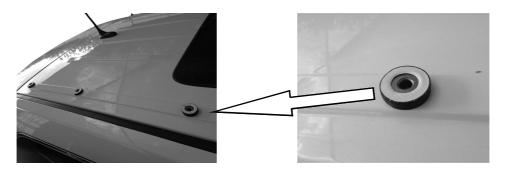
Place the Foot Rails onto the vehicle's roof, lining up the mounting holes in the bottom of the Foot Rails with the bosses on the vehicles roof. The Product Sticker must go to the rear of the vehicle and must be facing outwards. Push the Foot Rails as far back as possible.
