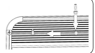
( **B** ) With your rack still upside down from Step 3A, slide a M8 x 20 Hex Bolt (Item 1) into the end of Slats 2, 3, 7 & 8.
