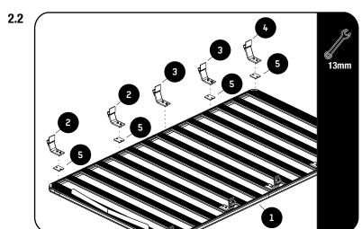
Loosely assemble the Legs & Spacers (Item 2, 3, 4 & 5) as shown, slats indicated in 2.2 using M8 Flat Washers and M8 Nyloc Nuts included in the Leg sets.
