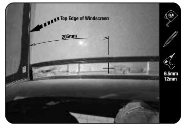
With the ditch mouldings removed, mark the middle of the ditch by measuring 205mm from the top edge of the windscreen.
