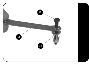
Insert the M6 x 30 Button Head Screw (Item 10) into the one side of the Jack Nut Tool (Item 11). Loosely fit a Jack Nut (Item 12) to the M6 x 30 Button Head Screw as shown. Using the Jack Nut Tool and a M6 x 30 Button Head Screw, insert the M6 Jack Nuts into all 8 holes. Place the assembly into the hole drilled. Using a Battery Powered Screw Driver and a H4 Allen Key Bit, set the Jack Nut into the hole while holding onto the handle of the Jack Nut Tool.
