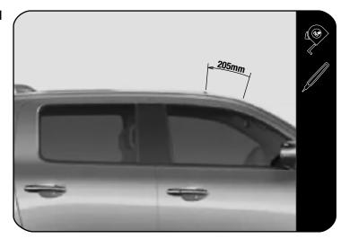
With the ditch moulding in place, mark the middle of the ditch moulding by measuring 205mm from the top edge of the windscreen shown in 2.3.
