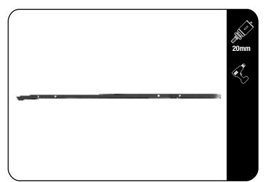
Unclip and remove the LH and RH ditch mouldings.
