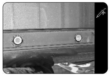
Place a bead of silicone around each of the Jack Nut openings inserted earlier in 2.4
