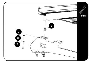
Fit your Roof Rack to the Foot Rails using M8 x 20 Hex Head Bolts, M8 Flat Washers and M8 Nyloc Nuts (Items 6, 7 & 8) as shown.
