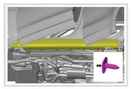
Remove the lower fixings of the Rear Rocker Panel Moulding
