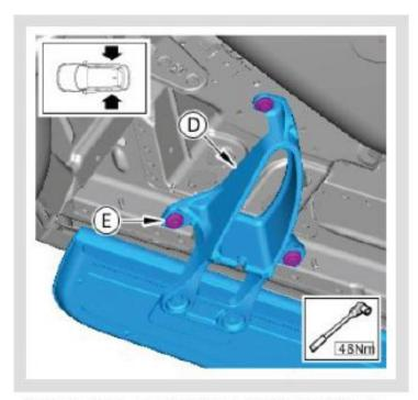
Tighten both the rear Side Step mounting bracket bolts. Torque: 48Nm.
