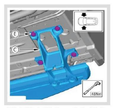
Tighten both the front Side Step mounting bracket bolts. Torque: 48Nm.
