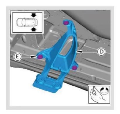
Install both rear Side Step mounting brackets.
