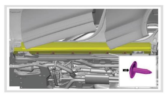
Install the lower fixings of the Rear Rocker Panel Moulding.
