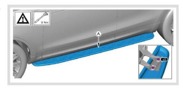
Tighten the Side Step mounting bolts.
