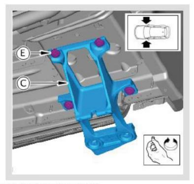
Install both front Side Step mounting brackets.
