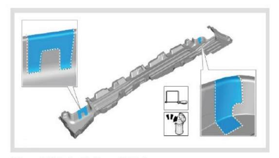
Using a suitable tool, cut the trims as illustrated. **Note:** Observe the cut marks on the trim panel. Repeat this step for the other side.
