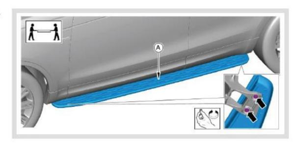
With the aid of another person, install the Side Steps. Note: Hand tighten only at this stage.
