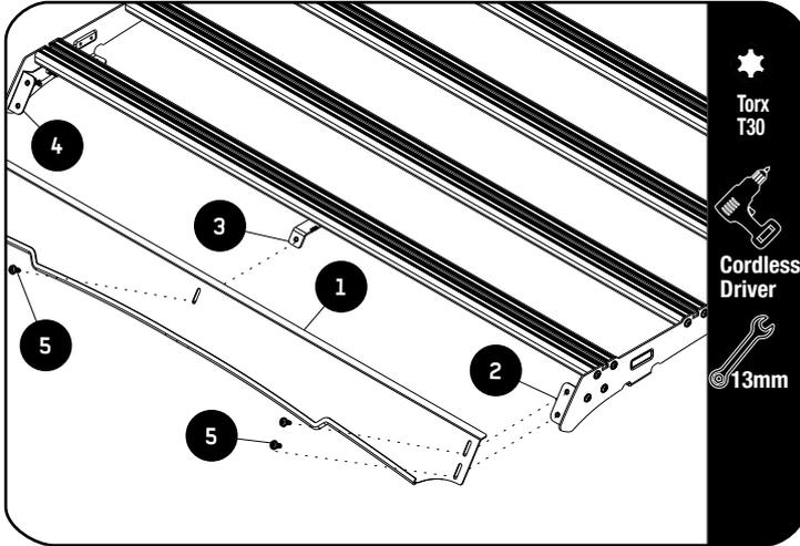
Assemble the Wind Fairing (Item 1) to the Support Brackets (Item 2, 3 & 4) using the M6 x 16 Button Head Flange Bolts using a T30 Torx as shown. Fully tighten the M8 Nyloc Nut that was inserted in 2.2.
