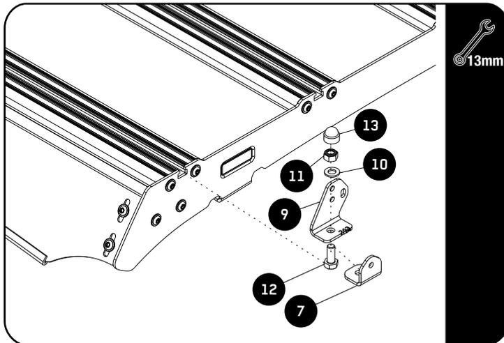
If you would want to fit a Light Bar with the Wind Fairing Slide the M8 x 20 Hex bolt (Item 12) into the Front Slat that was removed in 2.1 as shown, with the Light Bar Bracket (Item 7) assembled together with the M8 Flat Washer and M8 Nyloc Nut (Item 10 & 11) as shown and fully tighten. Place the M8 Nut Caps over the M8 Nyloc Nut (Item 10) Do the same on the opposite side.
