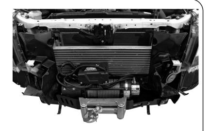
Fit the Rollers using the Nuts and Bolts supplied with your winch. If you have a Winch that is fitted with a Plasma Rope fit the supplied guide instead. You will need to unwind the Cable or Rope to feed it through the Rollers or Guide.
