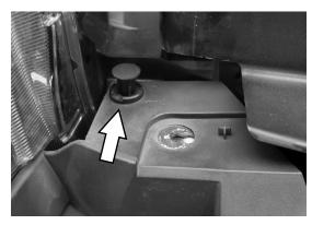
(D) On the edge of the wheel arch there are Screw-in studs. Use a Star/Philips screwdriver to unscrew. Once unscrewed pull out the Stud.
