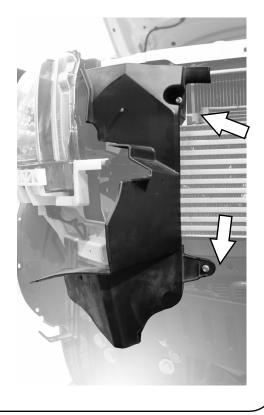
( H ) Remove the Front Chassis Member using a 15mm Socket wrench. Keep the Bolts for reuse in the next step.
