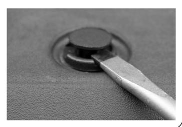
(B) Lift up the cover to see where the clips are located. From under the vehicle unclip the clips closet to the lights. You will be able to unclip the other clips from the top now.
