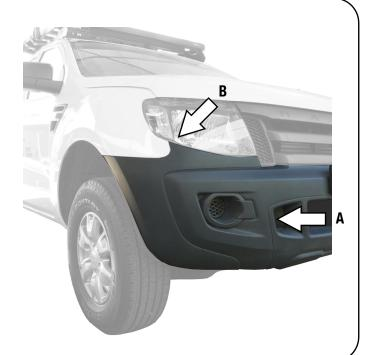
(G) Remove the Radiator Cowlings with an 8mm Socket Wrench, repeat this for both the Right and Left hand side of the vehicle.
