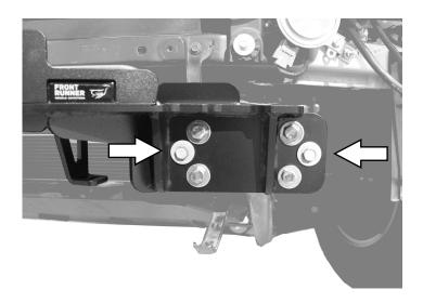
(B) With the Winch Plate in place reinstall the two Radiator Cowling's, using the four original 8mm bolts. See Step 2G for how it was removed.
