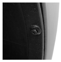
(  ${\bf E}$  ) Unscrew the bottom lip of the Bumper from the supports using 10mm Socket Wrench.
