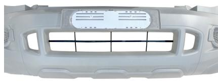
Using your Craft Knife cut the Ribs away. Cut as close as possible to the face of the Bumper to achieve a clean installation.
