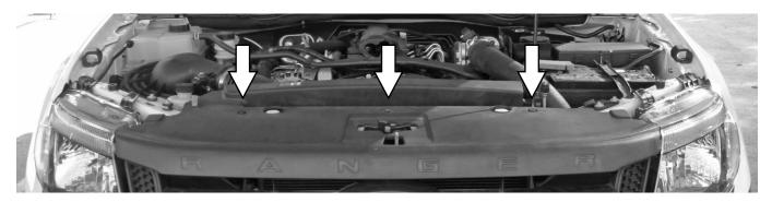
To remove the Press-in Studs use a medium 4 to 5mm wide flat screwdriver. Carefully place the screw driver under the head of the Stud and leaver up. It will not pull out all the way so be careful not to force it. With the head partially up remove the Stud. Repeat this with the remaining two Studs.
