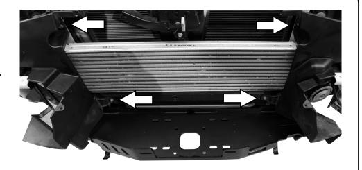
(C) Temporally install your Winch to check whether there is enough clearance between the Winch and the hydraulic pipe. If you find that the pipe is in the way, bend it slightly back toward the radiator. Check the assembly again to see that there is sufficient clearance. If happy move on.
