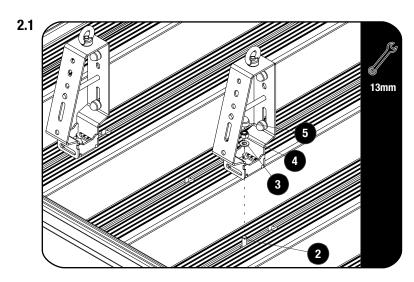
Secure the Roof Rack Accessory Mounting Bracket (Item 1) to your roof rack using fasteners supplied.
