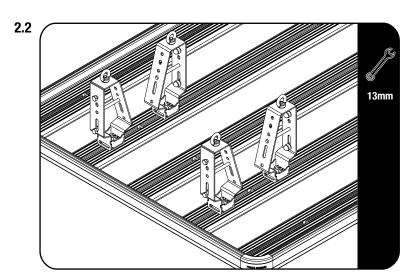
To transport BULKY cargo, use two pairs of Mounting Bracket.
