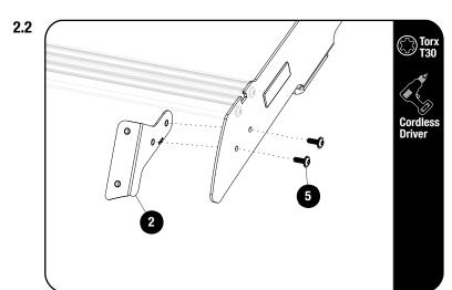
Assemble the Side mount Bracket (Item 2) to the Foot Rail using the M6 x 16 Button Head Flange Bolt (Item 5) and fully tighten.
