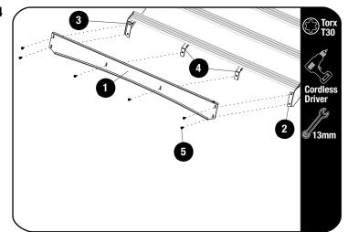
After the Rubber strip is fitted to the Slimsport Wind Fairing lift the Wind Fairing into place and fit the Wind Fairing to the Side mount Bracket (Item 2 & 3) using the M6 x 16 Button Head Flange Bolt (Item 5). DO NOT FULLY TIGHTEN.
