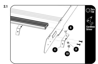
Starting by removing the 4 x M6 x 25 Thread forming screws from the front of the Roof Rack.
