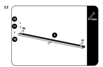
Fit the Light Bar Bracket 01 LH / RH (Item 4) for for Front Runner 40" Light Bar, using M8x16 Hex Bolt & M8 Nyloc Nut (Items 10 & 11). Fit the Light Bar and center on slat before fully tightening the brackets.
