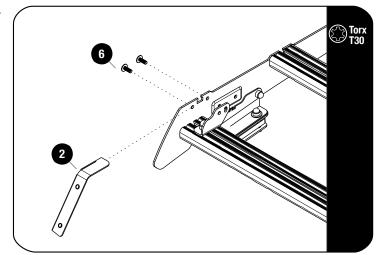
Secure the Wind Fairing Side Supports LH / RH (Item 2) to the foot rails top holes as shown using M6x16 Flange Button Head (Item 6).
