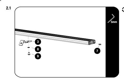
Slide one M8 Thin Nut (Item 7) into the T-slot of the front slat. Center the mid support bracket in the middle of the slat and secure using a Schnorr Washer and M8x12 Button Head (Items 8 & 9). Fully tighten.
