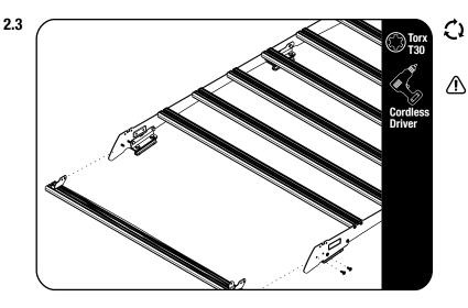
Secure assembly 2.2 to the front two bottom holes on the foot rails using the fasteners supplied with KSTH002
