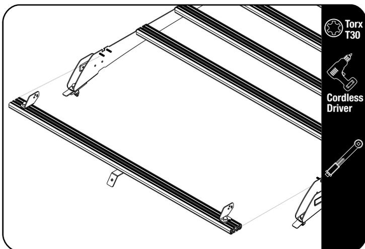
Secure assembly 2.2 to the front two top holes on the foot rails using the fasteners supplied with KSFR005.
