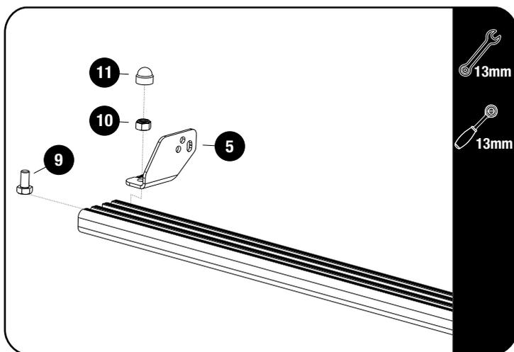
Fit the Light Bar Bracket 01 LH / RH (Item 5) for the 40" Light Bar, using M8 x 16 Hex Bolt & M8 Nyloc Nut (Items 9 & 10). Fit the light bar and center it on the slat before fully tightening the brackets.
